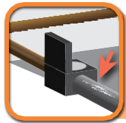
Water Service Line May be made of lead, copper, galvanized steel or plastic.
