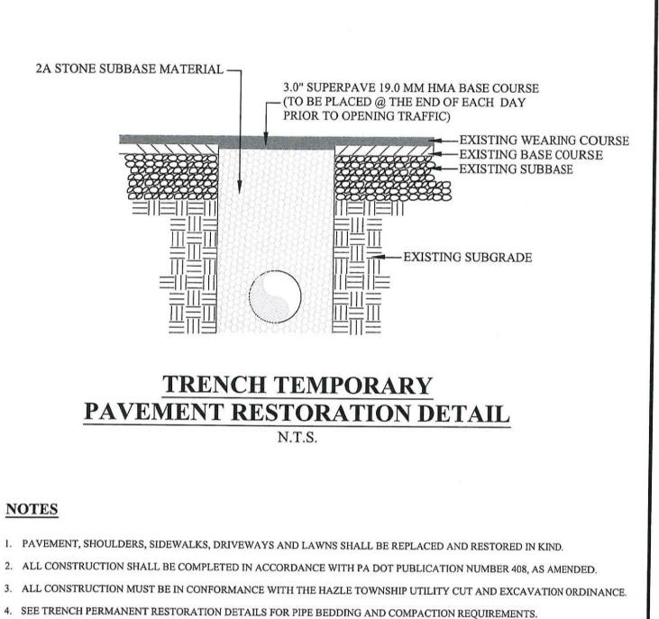
5. COLD PATCH IS NOT A PERMITTED MATERIAL FOR TRENCH TEMPORARY ROAD RESTORATION WITH THE EXCEPTION OF
